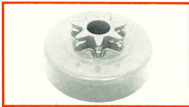
Worn chain sprocket
