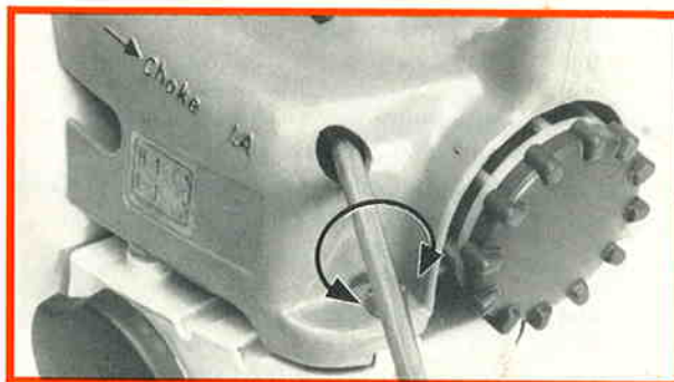
Regulating idle speed adjusting screw
