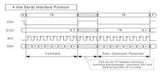
CSX is a slave chip selection, and the chip will only be enabled when CSX is at low
