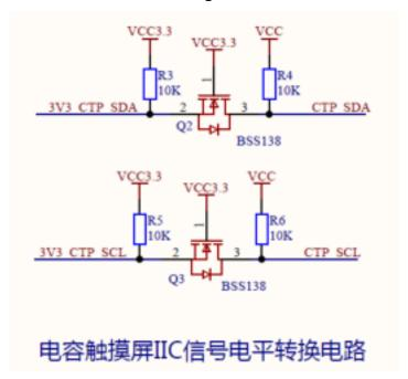
R3, R4, R5 and R6 are pull-up resistor, and Q2 and Q3 are BSS138
