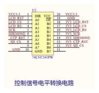
U2 is a level conversion IC that converts between 5V and 3.3V. This circuit only uses the one-way function of 5V to 3.3V, and the signals that the module needs to write are converted through this circuit.
