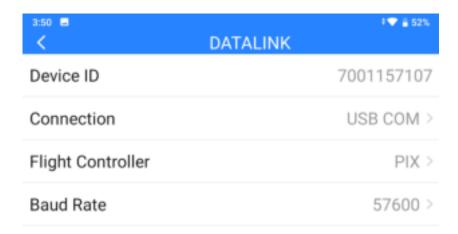
2. Run QGroundControl, go to "Application Settings – Comm Links" and "Add" a new connection. Name it as "USB-COM". Connection "Type" as "Serial". Match the baud rate.
