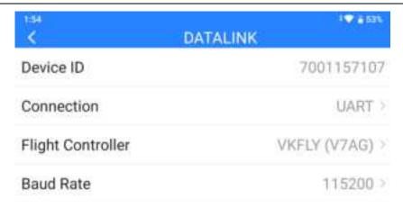
Run VK GCS, remote controller will communicate with the VK app automatically and shows "device connected". Datalink connection is established.
