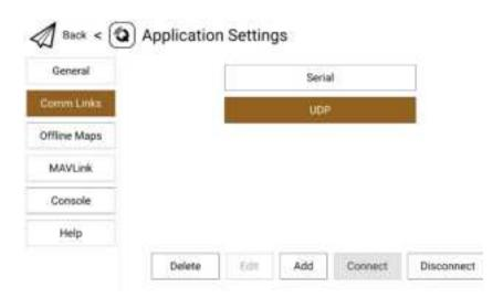
5. Confirm and start to "Connect". The top progress bar in QGC starts to move, which means the remote controller is communicate with QGC automatically. Please wait until the datalink connection is established.
