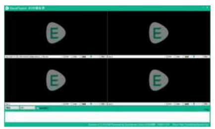
4. Input the complete RTSP addresses of the connected camera or gimbal in Easyplayer to display the video stream.
