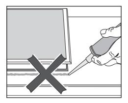
⚠ Damage caused by incorrect installation.
