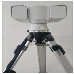
Adjust the position of the scanner with Mount Plate until the center hole of the Mount Plate is aligned with the center hole of the Tripod.
