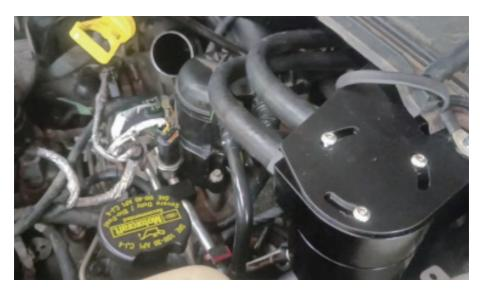
**Step 26:** Reinstall the hot-side intercooler pipe. (1x worm gear clamps, 1x spring clip) Congratulations! You have finished installing the 2011-2016 Ford 6.7L Powerstroke CCV Reroute/Delete w/Catch Can Internal External Kit
