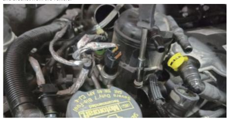
Step 5: Remove the bolts that secure the fuel rail. (2x 8mm bolts)
