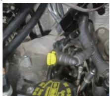
Step 15: Install the CCV adapter and aluminum plug.
