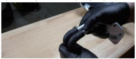
**Step 12:** Grease the O-ring groove on the aluminum adapter and place the thin o-ring within the groove.
