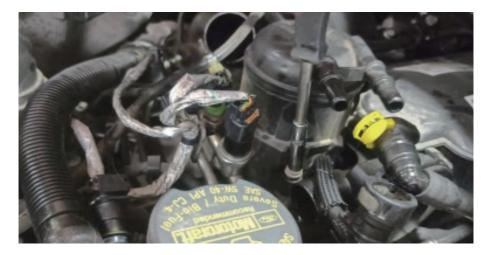
Step 7: Lift the air-oil separator and clean the housing.
