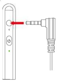
Connect the earset to the Audio port in the device.
