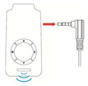
Removing the earset from the device makes the speaker produce sound.
