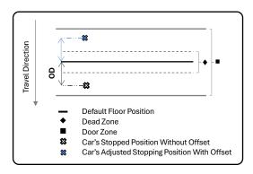
Offset Down [OD] = Default Floor Position - Car Position After Stopping
