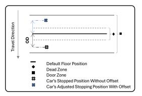
Offset Down [OD] = Default Floor Position - Car Position After Stopping
