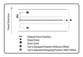
Offset Up [OU] = Car Position After Stopping – Default Floor Position
