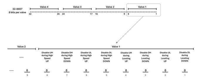
Step 1: Replace 0 with 1 to disable the required valve commands for valve 1
