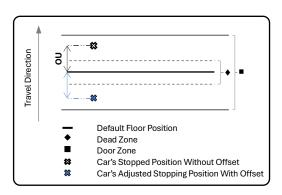
Offset Up [OU] = Car Position After Stopping – Default Floor Position
