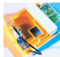
Sound Guard™ III Proprietary Compression Driver Protection Circuit.
