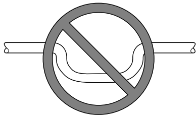
Fig. 15 – Insufficient Condensate Trap
