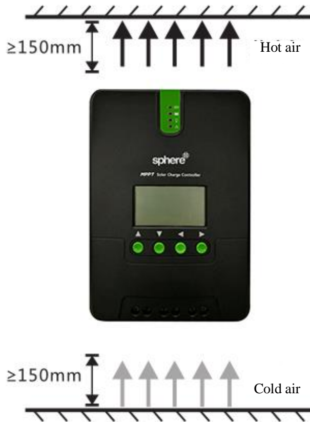
Fig. 2.1 Installation and heat dissipation
