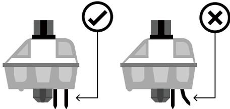
Before installing switches, be sure the pins are clean and straight.
