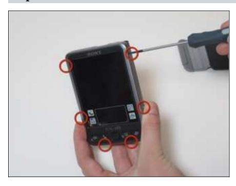
• Remove the six screws holding the outer case of the Sony Clie.
