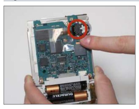
Remove the two screws holding the scroll wheel.
