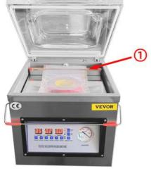
6.MARINATE: Click the marinate button in the upper right corner of the control panel, the marinate indicator light will light up, adjust the pumping time, and start the marinate work. At this time, the machine is in a vacuum only state without sealing.
