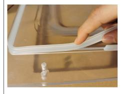
2. Replace the Chamber Sealing Strip with a new one
