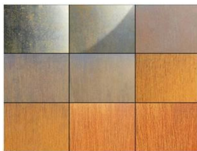
The Corten Steel weathering process
