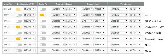
If using DJI remote control, turn on UART4 RX and turn off UART1 RX, Set the receiver protocol to SBUS
