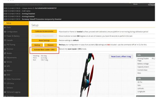
2/ BF Configurator will display to enter DFU mode. If it does not enter DFU mode, it may be that the driver is not installed. The driver can be installed using IMPULSE RC software
