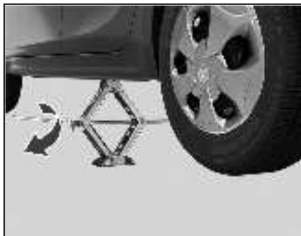
Lifting the front wheel using jack
