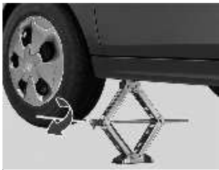
Lifting the rear wheel using jack
