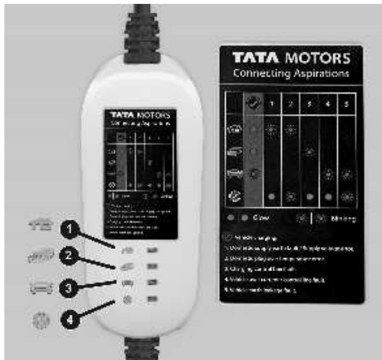
Slow charging control box
