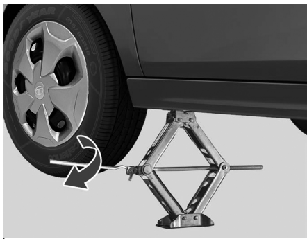
Lifting the rear wheel using jack
