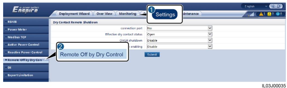
Figure 6-39 Remote Off by Dry Con
