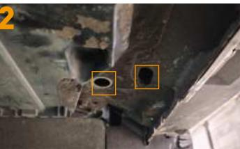
Place the pin "1" & "2" into the factory mounting holes.
