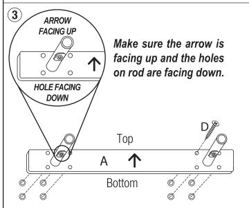
**Step 3:** Insert wall screws (D) through wall mount (A) and into placed wall anchors (C) and secure with screwdriver (H).
