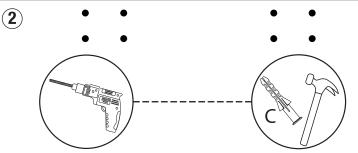
**Step 2:** Drill holes into all the marked areas with the twist drill bit. Then knock all wall anchors (C) into place with hammer.
