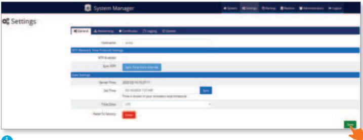
During initial setup, make sure that the AC-HOST has a network connection, and that either NTP is set to NTP Enabled, or click
