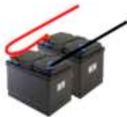
Figure 4: Recommended wiring for connecting batteries in parallel.
