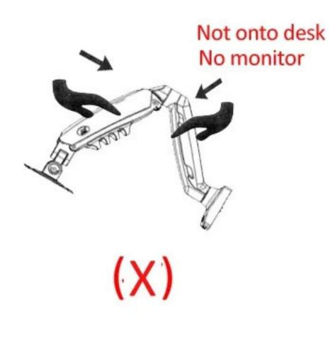
3. Question: the torque adjust hole is not able to reach Answer: first, finish the instal and attach monitor onto the mount, se press the arm down, then the hole will come out
