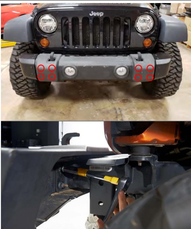
(Fig 3) From under the vehicle, access and remove the (8) 18mm nuts securing the factory bumper to the vehicle.
