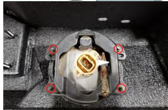
(Fig 6) Install the fog light using (6) M4 Bolts, (10) M4 Flat Washers, (6) M4 Lock Washers, and (4) M4 Nuts. Repeat the process for both fog lights.
