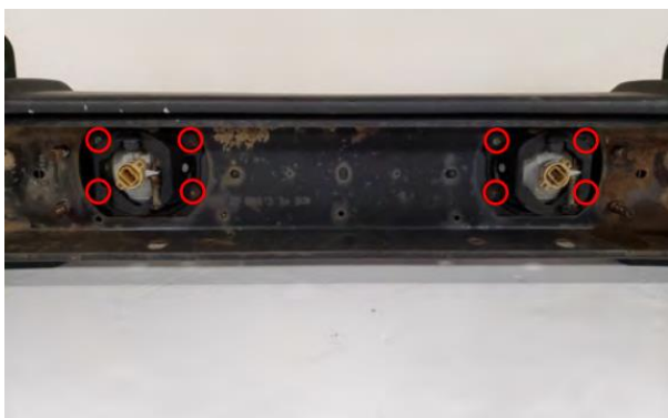
(Fig 5) Remove the (8) 7mm screws securing the fog lights to the factory front bumper.
