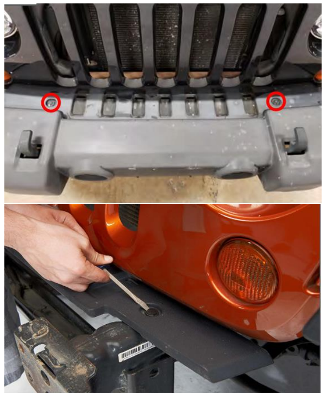
(Fig 4) Remove the 2 push pins holding the top cover onto the vehicle.
