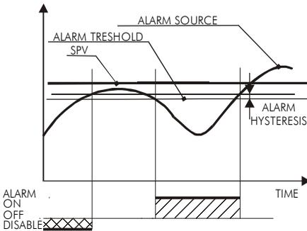
This alarm is disabled at the starting of PL300 and it is automatically activated when the alarm source exceeds the alarm treshold of a value which is equal to the hysteresis. Then the alarm works like the above described “deviation low alarm”.
