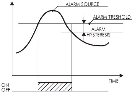
Max. treshold for the alarm source (one of the analog inputs).
