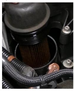
**Step 2:** Ensure that the threads on locking cleat are aligned with threads on adapter body prior to install. (as shown)
