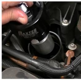
**Step 4:** Lubricate the 1/8" hex plug and install in unused port.
