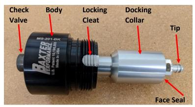
**Step 3:** Lubricate the face seal on the docking collar (body and tip O-rings will be installed later). Install the Adapter until it bottoms out, then back it out less than 180 degrees to expose an NPT port to be utilized for the Schrader valve. Note the orientation (the opposite one will be plugged with the included hex plug) and remove adapter.
