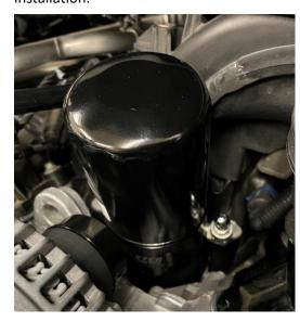
Servicing instructions at Oil Change: Prior to draining engine oil from oil pan, and oil filter removal, apply minimum 30 PSI to the Schrader valve for at least three seconds. This will evacuate the oil retained in the oil filter and cooler. Then, remove oil filter and replace.
