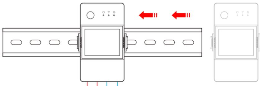
First fix the guide rail at the position where the equipment needs to be installed, and then slide the device base buckle against the side of the guide rail.
