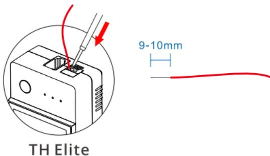
Press the white button on the top of the wire connecting hole to insert the wire corresponding, then release.
