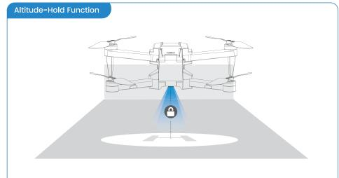
The drone is designed with an altitude-hold function to maintain its altitude after releasing the left joystick. (The left joystick will automatically spring back to the middle)
