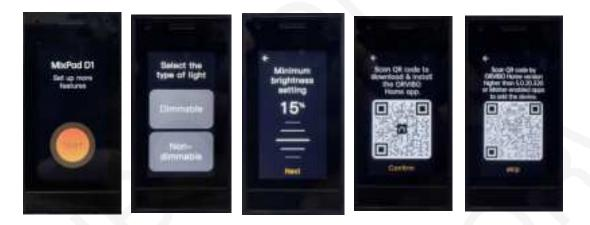
• If the device skipped the setup process or has already joined the ORVIBO Home app: Navigate to the "Settings" page of MixPad D1 and tap on "Add to App".
