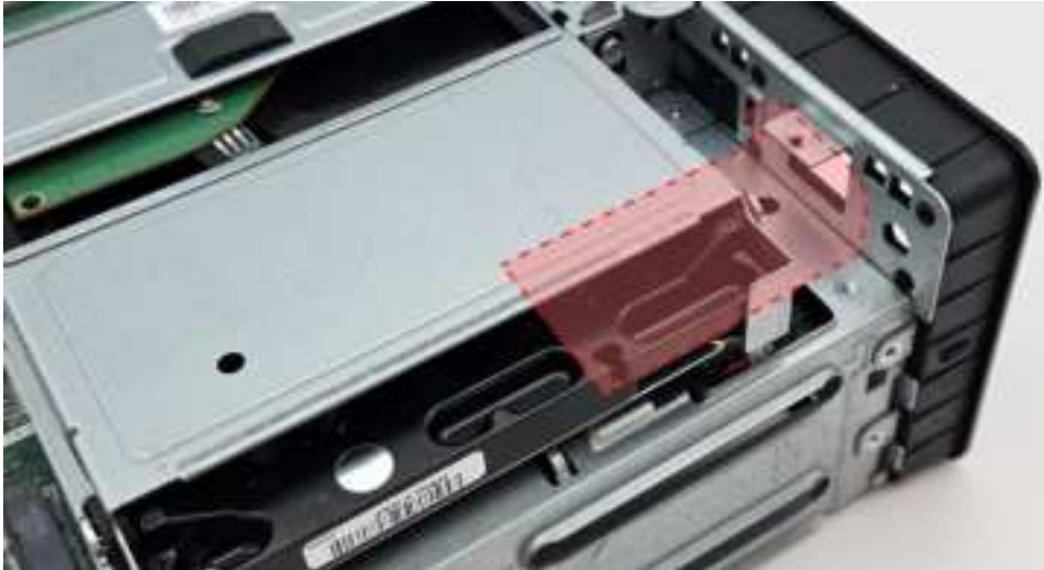
Figure 10, P3 Ultra SFF Gen 2 HDD & TBT interference (TBT in red)
