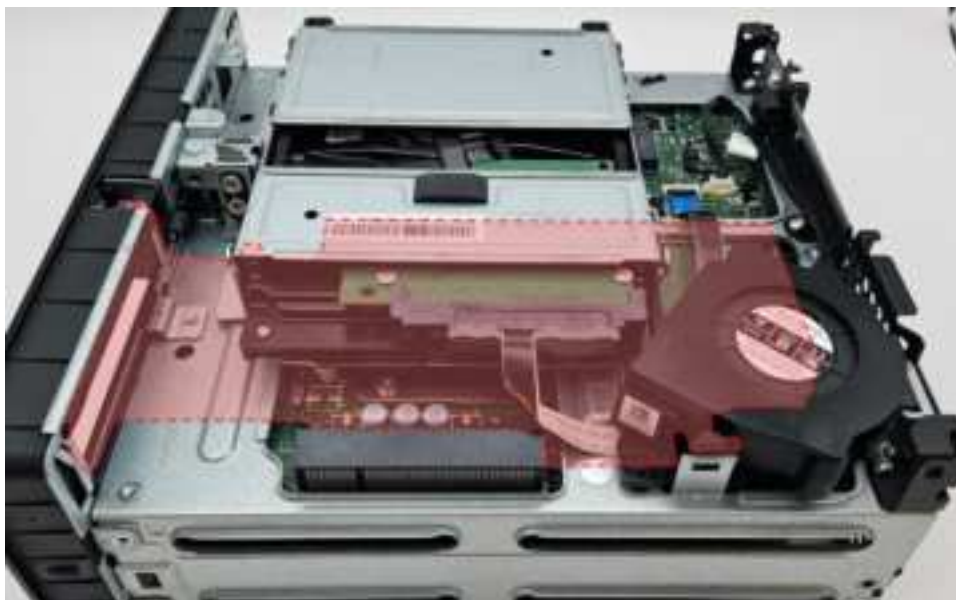
Figure 11, P3 Ultra SFF Gen 2 HDD & x8 slot interference (A400 in red)
