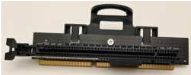
Figure 5, Double Riser Card (FRU# 5C51M21374).
