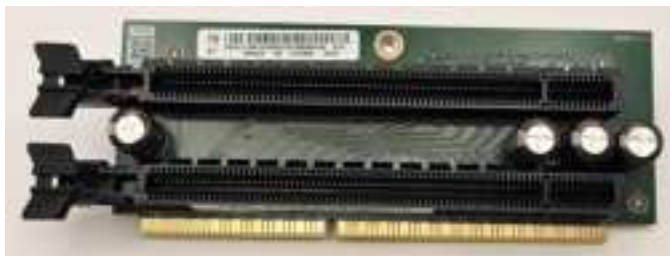
Figure 5, Double Riser Card (FRU# 5C51M21374).
