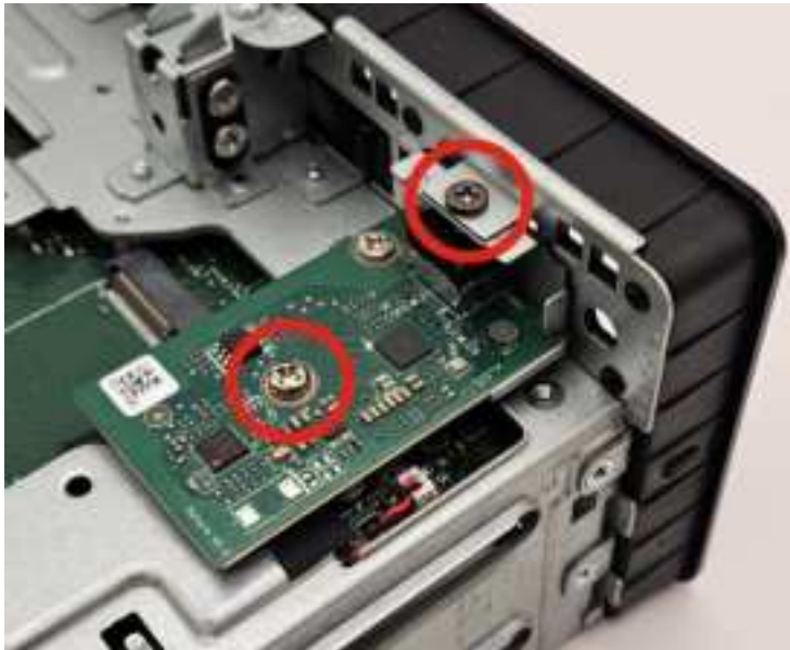
Figure 7, P3 Ultra SFF Gen 2 Thunderbolt BTB Installed with Screws
