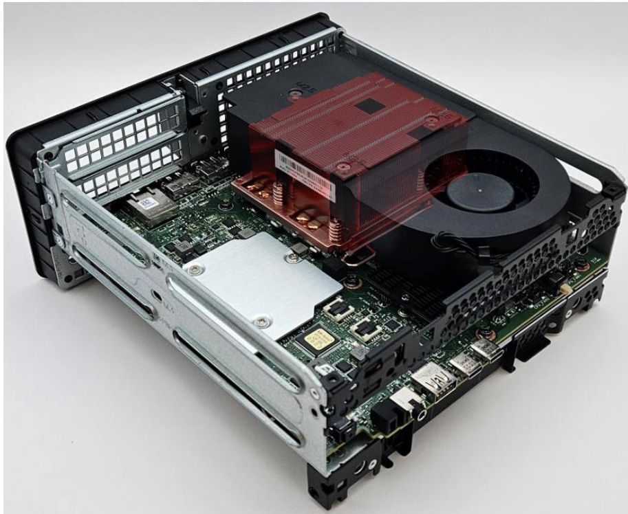
Figure 8, P3 Ultra SFF Gen 2 with 65W heatsink (fins highlighted red)
