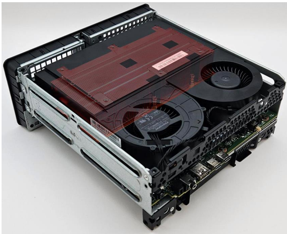
Figure 9, P3 Ultra SFF Gen 2 with 125W heatsink (fins highlighted red)
