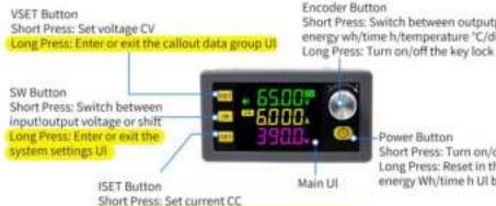
Short Press: Switch between outputpower w/capacity Ah/ energy wh/time h/temperature "C/display in rotation
