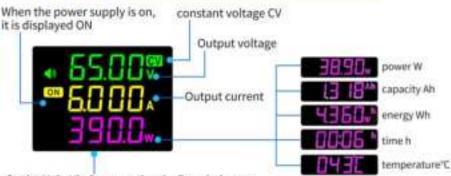
On the Main UI, short pressing the Encoderbutton toggles between displaying outputpower (W), capacity (Ah), energy (Wh), time (h), temperature(c), showing themin rotation.
