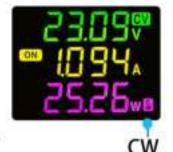
When the constant power function is not turned on, the power supply only has the functions of constant voltage (CV) and constant current (CC), which automati-cally switch based on the load;
