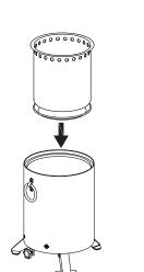
3. Place the log grate into the chamber for combustion
