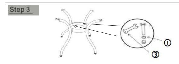
Repeat Step 2 to attach the remaining 3 Legs(B) to the Support Ring(C).
