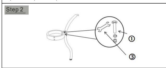
Loosely affix the Support Ring(C) to Table Leg with pre-attached Levellers(B) using Washers, Spring Washers, and Hex Bolts(①), with the Spanner(③).
