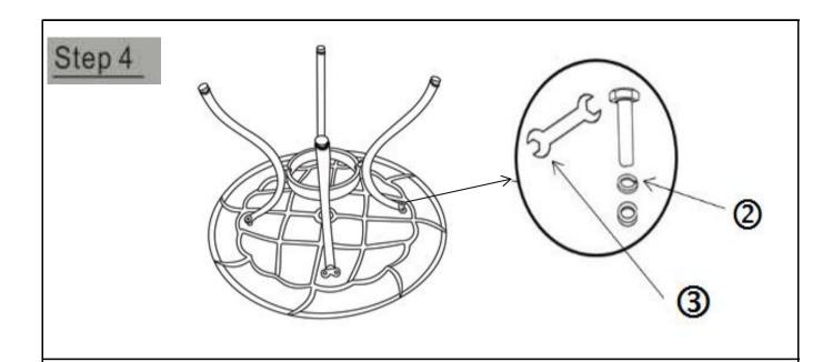
Lay the Table Top(A), facedown, onto a flat, soft, clean surface. Attach the Table Legs(B) to the Table Top(A) using Washers, Spring Washers, and Hex Bolts(2) with the Spanner(3).
