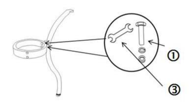
Loosely affix the Support Ring(C) to Table Leg with pre-attached Levellers(B) using Washers, Spring Washers, and Hex Bolts(①), with the Spanner(③).
