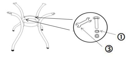
Repeat Step 2 to attach the remaining 3 Legs(B) to the Support Ring(C).
