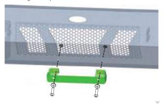
Install the bumper to the vehicle using the factory nuts. Repeat this step for the opposite of the bumper. Adjust the bumper to the desired location. Tighten up all bolts.
