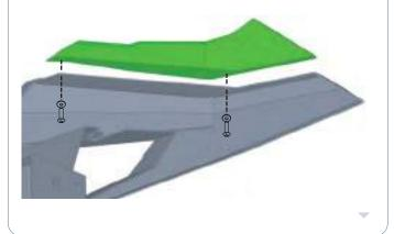
Install the license plate bracket to the bumper using the (2) M8x20mm button bolts, (2) M8x20x1.5mm flat washers, (2) M8 flange lock nuts. Tighten up all bolts.
