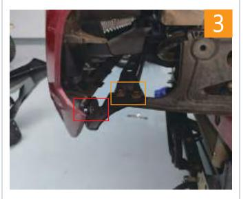
Stick the EVA to the bumper and install the left wing to the main body using (3) M10x25mm hex bolts, (3) D10 lock washers, (3) M10x25x2mm flat washers. Repeat this step for the opposite
