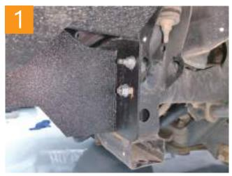
Install the skid plate to the bumper using the (4) M8x20mm button bolts, (4) M8x20x1.5mm flat washers. Do not tighten the hardware at this time.
