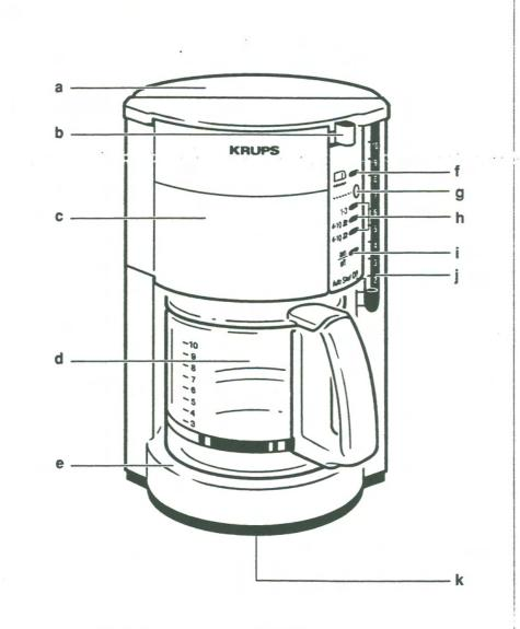
a: Hinged water chamber lidb: Release buttonc: Swing away filter holderd: Glass-Carafe
