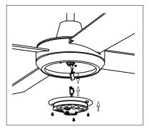
Carefully install the glass shade into the main body and turn it clockwise to lock it.
