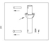
Insert the down rod into the motor housing's hole and turn it in order to align the holes on both sides with the holes on the down rod.
