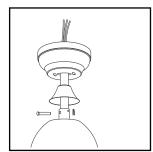
If screws are not properly tightened, the motor might oscillate. This could be dangerous.
