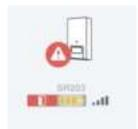
When the cover of the SR203 is removed, the tamper icon (hammer) is displayed as below.
