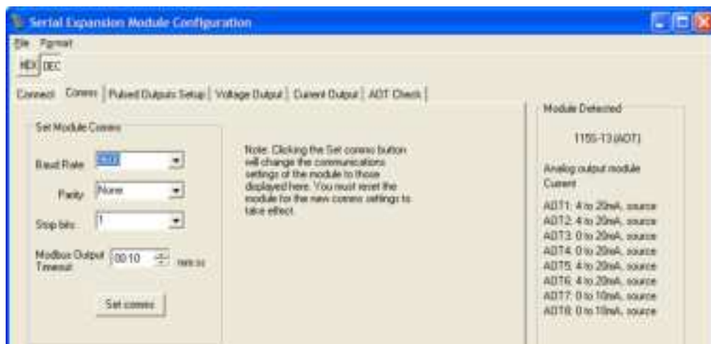
Figure 4-2: Communications configuration screen.
