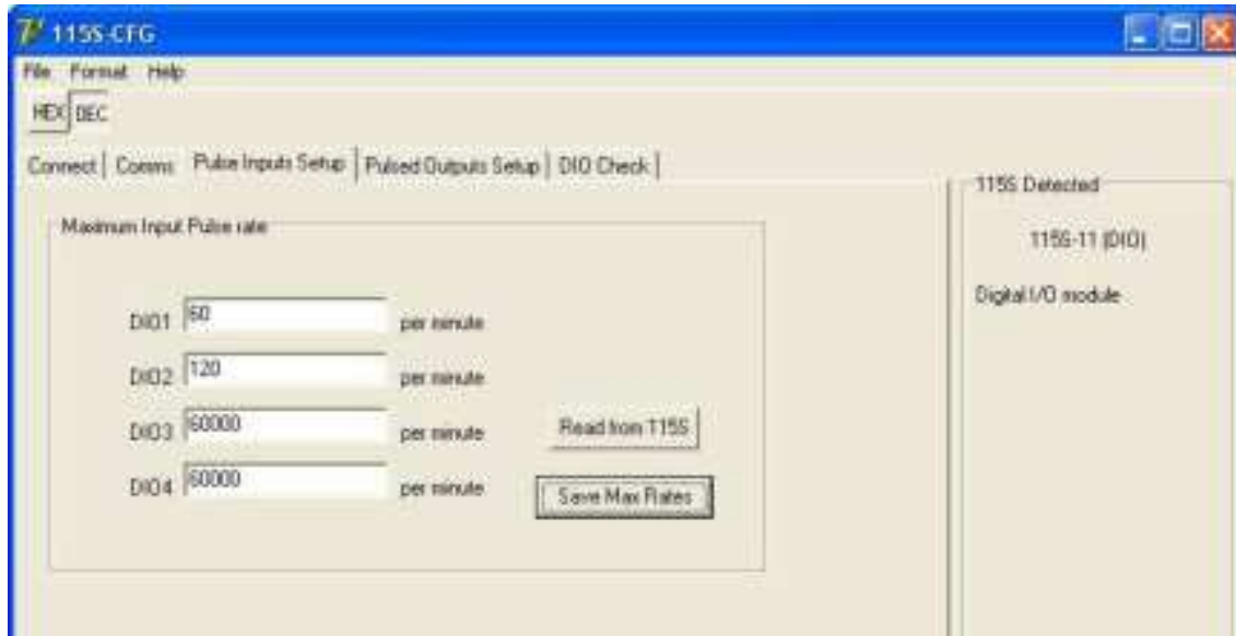
Figure 4-4: Pulse inputs setup. Only available on a 115S-11 module.
