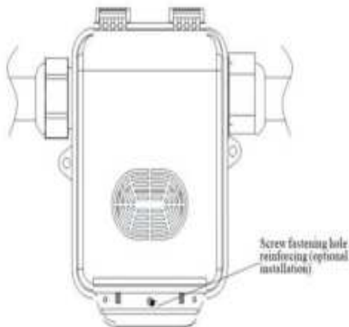
Fig.4 Fastening screw installation position
