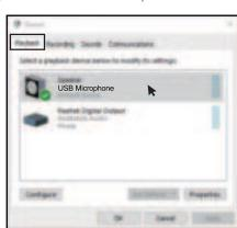
(2) Double click the speaker ("USB Microphone") is being used>>Properties>>levels>>drag progress bar to adjust volume of output.
