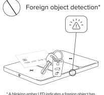
\* A blinking amber LED indicates a foreign object has been detected (metal objects like keys, coins, magnets, etc.) and the device is automatically turned off to ensure safety. Removal of foreign object and proper alignment of phone will result in normal operation.
