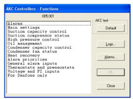
The operation is divided up into several function groups. When a selection has been made, push "OK", and you may continue to the next display. By way of example, "Suction capacity control" has been selected here.
