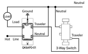
Note: For 3-way configurations, ensure the smart dimmer is installed in the junction box where Line (Hot) enters the electrical circuit. Insert wires into holes, do not wrap wires around screws. Do not remove screws. The Qoralux 6 Button keypad Dimmer is designed to operate in either 120VAC or 277VAC circuits. For 277VAC 3-way circuits, use standard "off-the-shelf" 277VAC compatible 3-way switch.
