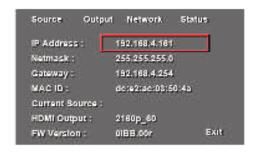
Open the browser and input the IP address, e.g. 192.168.4.161, to access the login interface.
