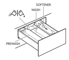
PREWASH - Compartment for prewash phase, soak programme or stain remover. The prewash and soak detergent is added at the beginning of the wash programme WASH - Compartment for washing phase. SOFTENER - Compartment for fabric softener and other liquid treatments (fabric conditioner, starch).
