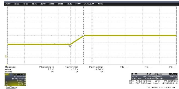
Figure 37: 9V→15V Rise Time = 79.0ms
