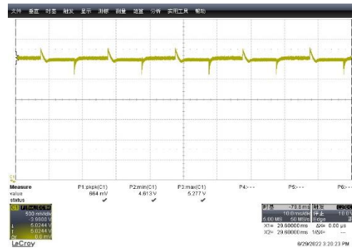
Figure 29: 264Vac/50Hz Port-C@ Vout=5V
