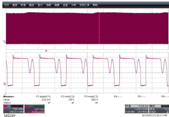
Figure 16: Q1 Vds Voltage stress
