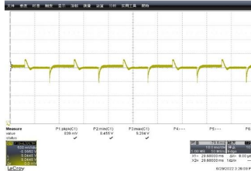
Figure 31: 264Vac/50Hz Port-C@ Vout=9V
