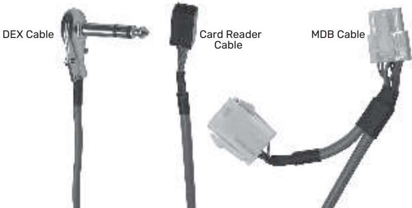
FIGURE 7 G11 TELEMETER CABLES
